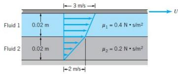
**P4.** Determine the magnitude and direction of the shearing stress developed on the plate. Express your answer in terms of U and  $\delta$  (the fluid is Newtonian).
