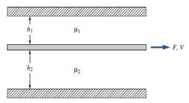
**P3.** Let two layers of fluid be dragged along by the motion of an upper plate as shown in Fig. P5. The bottom plate is stationary. The top fluid puts a shear stress on the upper plate, and the lower fluid puts a shear stress on the bottom plate. Determine the ratio of these two shear stresses.
